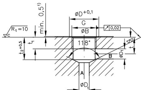
1) If pressure exceeds 100 bar at B, sinking is required!
